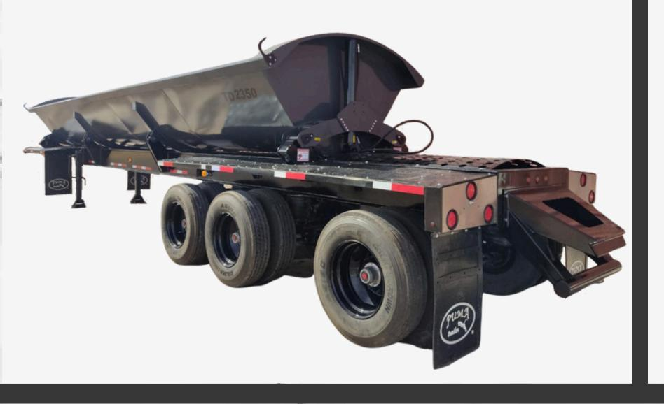
Instantaneous air exhaust-height control valve Any color combinations for paint job (10) 24.5 x 8.5 steel wheels with radial tires.
